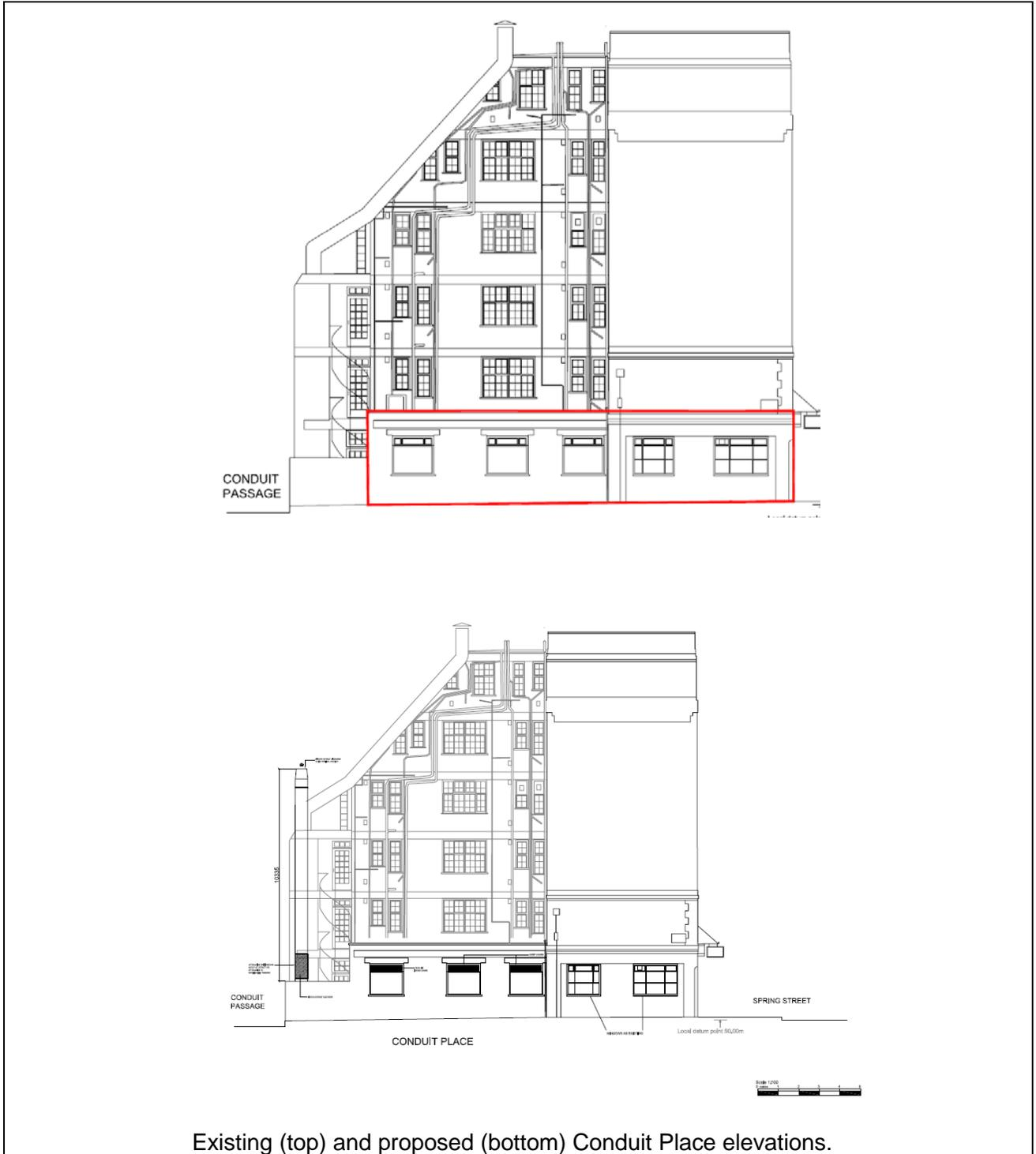
Existing (top) and proposed (bottom) Conduit Place elevations.
